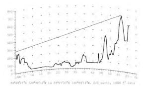
Figure 11. Vandenberg uplink to Cuesta Peak terrain profile. Path is 61.3 km bearing 347°T. Profile extends 5 km past the ENG-RO site.
