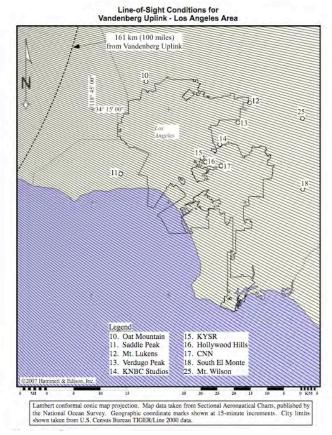
Figure 5. Shadowgraph showing line-of-sight conditions for the Vandenberg uplink antenna in the Los Angeles area.
