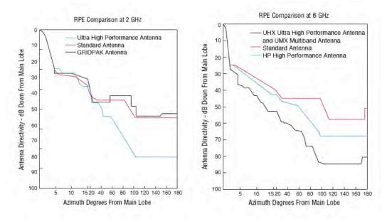
Figures 8 (left) and 9 (right). RPEs for Andrew Corporation standard performance, high performance and ultra high performance parabolic antennas at 2 GHz and at 6 GHz. These figures are courtesy of Andrew Corporation.
