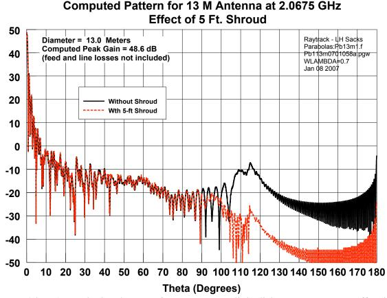
Figure 7 (above). Calculated RPE of 13-m USB uplink dish, zero to  $\pm 180^{\circ}$  off axis. Courtesy of The Aerospace Corporation (Preliminary).
