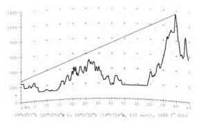
Figure 10. Vandenberg uplink to Broadcast Peak terrain profile. Path is 59.7 km at 123°T. Profile extends 5 km past the ENG-RO site.
