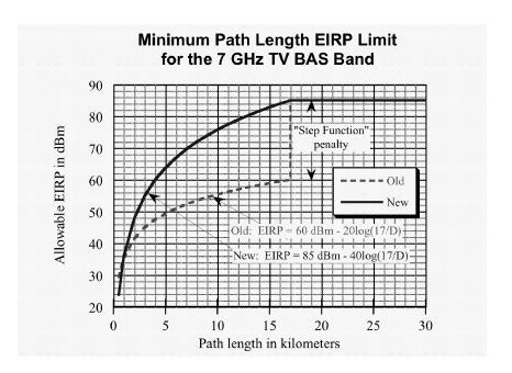
Fig 5. New vs old EIRP derating formulas for 7 GHz TV BAS links. Similar formulas apply at 13 GHz.
