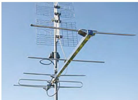
Fig. 4: Author's hybrid VHF high-band/UHF antenna combination is lightweight and wasn't too difficult to install. The pre-amp is mounted between the two antennas.
