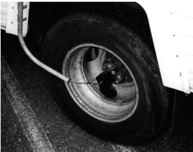
**Figure 4.** Optical shaft encoder installation.
