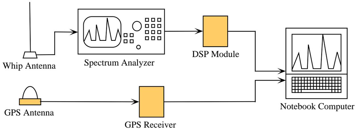
**Figure 1.** Block diagram of spectrum analyzer recording system.
